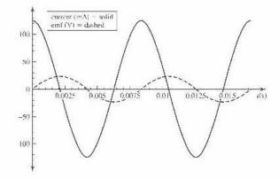
b) ε<sub>max</sub> = 23.4 V; i = 0, since the emf and current are 90° out of phase.
